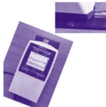
(b) Talysurf measuring instrument with Knob position
